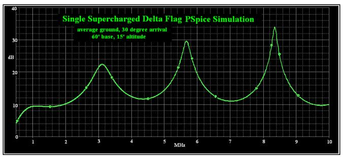
The length of the coax for these simulations is 100 feet. As the coax length is increased, the frequencies of the resonances decrease, and for 200 feet length the first resonance is about 1600 kHz.
