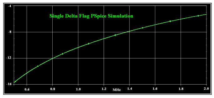
The simulation agrees with EZNEC to within 1 dB, assuming that the single flag antenna which EZNEC models is impedance matched to the receiver (which can easily be done with a broadband transformer). The PSpice schematic already includes impedance matching. This may be regarded as establishing the validity of the PSpice antenna simulation method for average ground and arrival angles in the neighborhood of 30 degrees.
